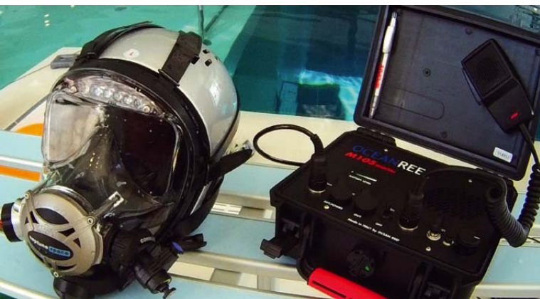
Fig 2. Full face mask-helmet combination with acoustic communication system (OceanReef Inc, photo: DAN Europe)
