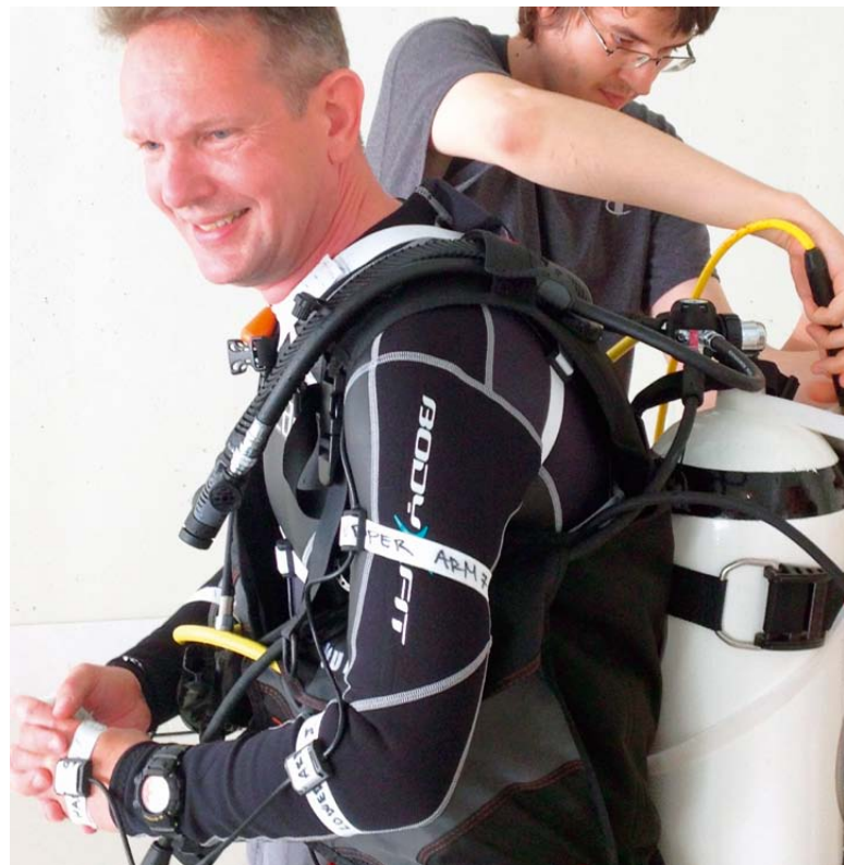
Fig. 4. DiverNet Sensors are mounted prior to the dive to test diver Robert van den Berg, DAN Europe Regional Training Coordinator, Austria. photo: DAN Europe
