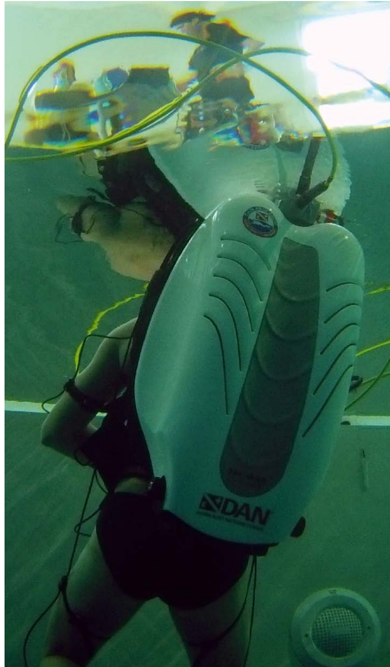
Fig 3. Diver with DiverNet sensors and redundant-protected SCUBA system (Innovasub LTD, photo: DAN Europe).
